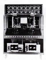
Two rear panels in the JH-16 cabinet fold down to provide access to the rear of the transport and the meter housing. The lower panel permits access to the transport connector panel and the reeling motors. Printed circuit bus boards in the meter housing reduce point-to-point wiring and facilitate re-lamping.
