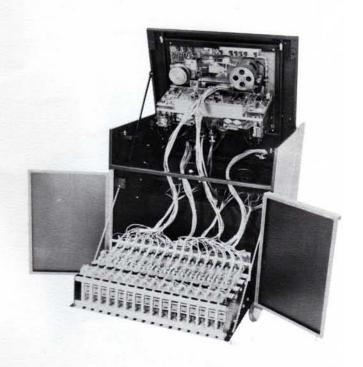
Both sections of the remote control are separately removable for ease of servicing. Overdub and safe-ready switches are P.C. mounted with easily removable plug-in lamps. Relamping is accomplished by removing the lower wrap panel. The Auto-Locator unit is self-contained and plugs into the function remote section.
