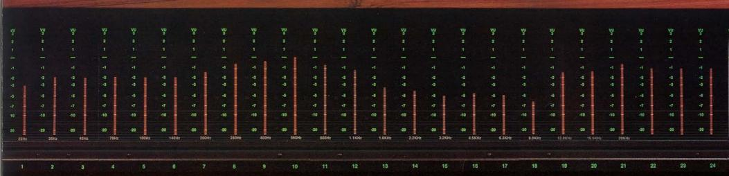
Plasma Display: High resolution 100-segment plasma displays can monitor audio or DC levels, and are switchable to either PPM or VU ballistics.
