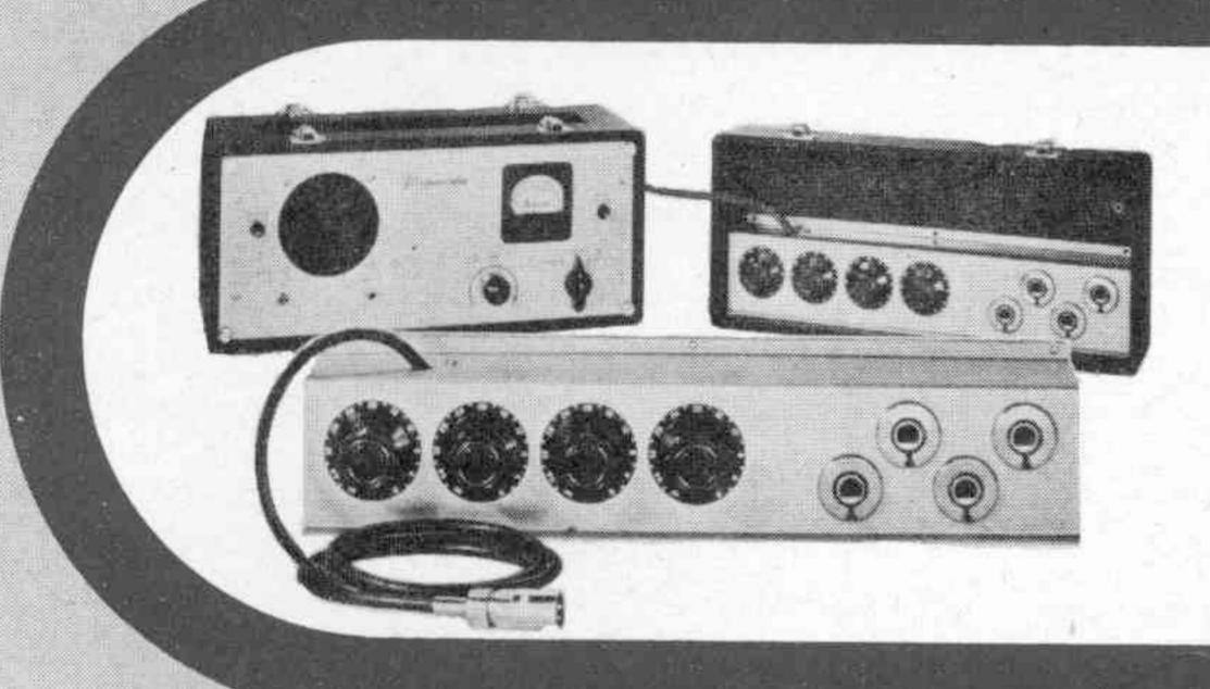
PT6-IM4... Multi-channel low level mixer for up to four 30/50 ohm low impedance microphones. Use with PT6-J or PT63-J single microphone input amplifiers. 17" long and mounts in amplifier case cover. Mixer plugs into microphone input on amplifiers. Gain-control on amplifier acts as master for all microphones. Uses 4 ladder type attenuators (2 db per step). Cannon receptacles and plugs. Weight: 3½ lbs.
