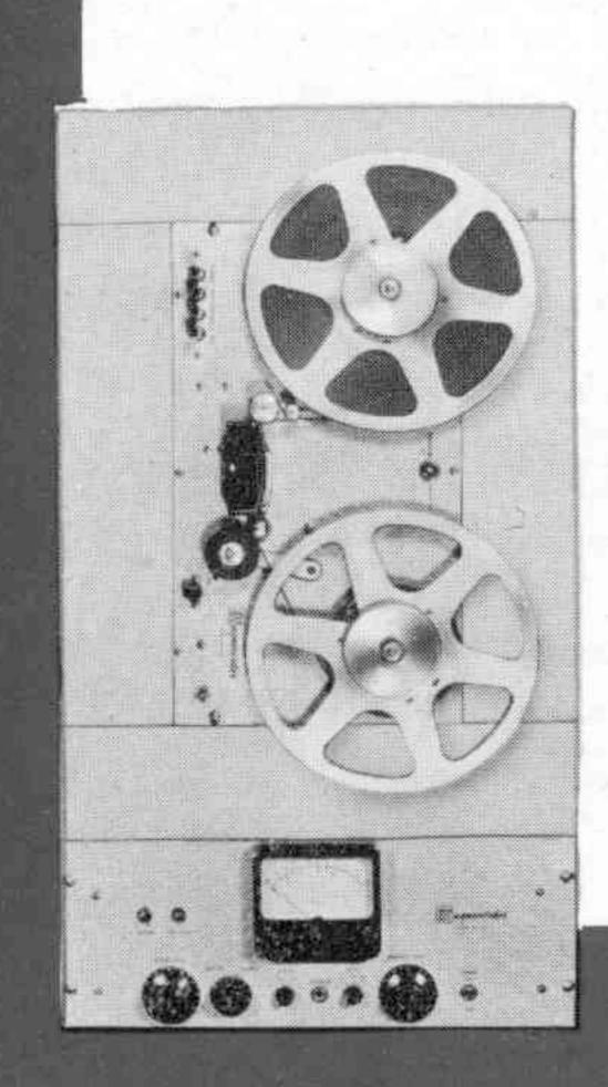
19" wide for direct mounting in Console Rack, or Portable. Input: 600 ohm, balanced—also bridging input. Output: zero level at 600 ohm, balanced. Switch for 7½" or 15"/sec. tape speed equalization. Switch for bias, record or playback reading on 4" illuminated VU meter. Complete with tubes—interconnecting cables are attached to PT7-A. 7"x 19" Gray hammerloid enamel finish. Weight: 26½ lbs.
