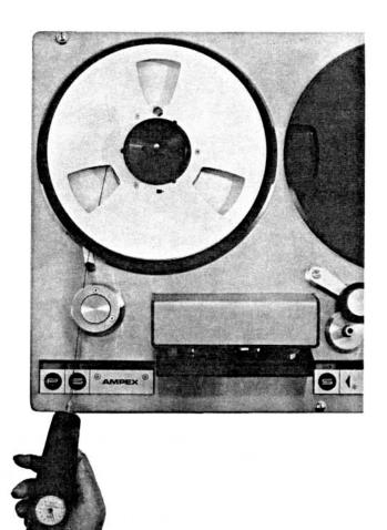
Fig. 4-2. Checking Holdback Tension
