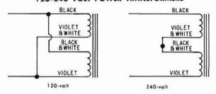
Stereo 70s supplied with power transformer PA-521 may be connected for either 120 volt or 240 volt AC operation as follows:
