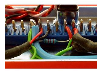
In situations where the **fader connection is not used** (most Neve 45 series consoles except BCM10's) then the resistor remains in place.
