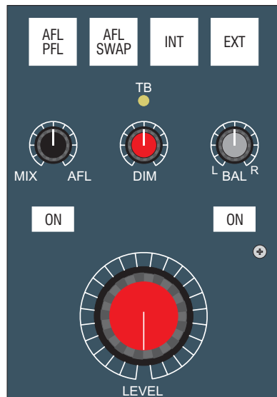
Control Room Monitor Level Controls
