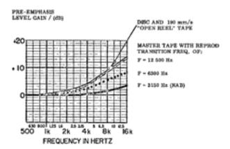
**Fig. 3** Recording pre-emphasis for master tape with different postemphasis transition frequencies F = 3150 Hz (NAB), 6300 Hz, and 12 500 Hz. Pre-emphasis used for disk recording and for 190 mm/s (7.5 in/s) open reel commercial tape records shown for comparison. See footnotes 3 and 4 for detailed conditions.
