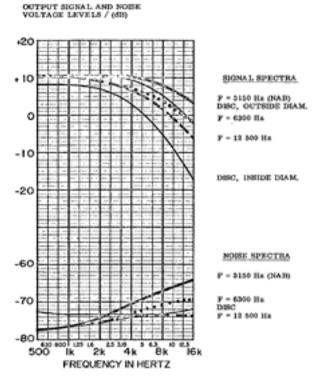
**Fig. 2** Saturation signal and  $\frac{1}{3}$ -octave noise spectra. Heavy curves: For a fourth-generation master tape with various reproducing transition frequencies F = 3150 Hz (NAB), 6300 Hz, and 12 500 Hz. Light curves: For a  $33\frac{1}{3}$  rev/min vinyl disk pressing. See footnotes 3 and 4 for detailed conditions.
