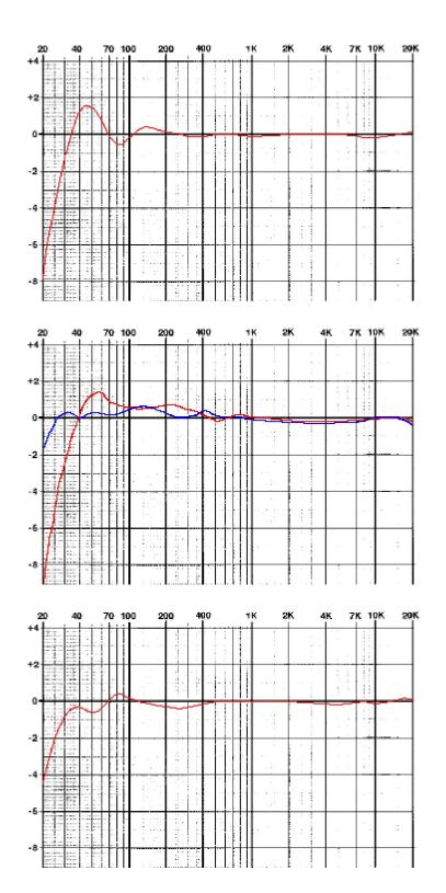
Studer A820 half-inch 2-track, 30 IPS. Very nice machine to mix onto if you don't mind the slight low end bump, which I don't. Also good at 15 IPS but I forgot to get a curve.
