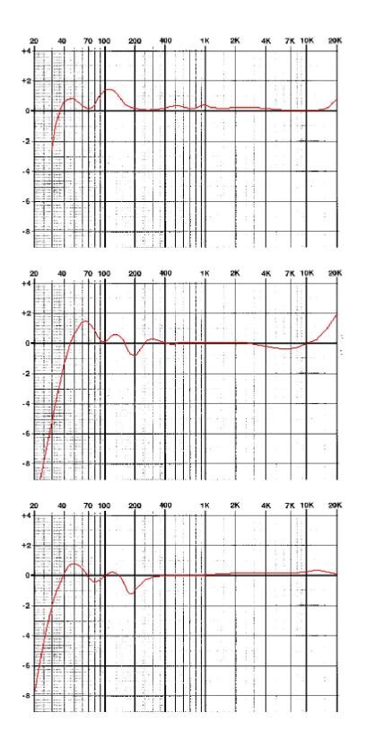
Studer A820 2-inch 24-track, 30 IPS. Slightly earlier generation than the 827 above; similar curve, but the bass roll-off is steeper. The peaks are a tiny bit further to the left though. Also a very good analog machine.
