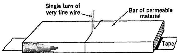
Fig. 2. Idealized bar-type ferromagnetic reproducing head.
