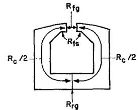
with sufficient accuracy; second, playing tape on such a head causes wear which changes the head's sensitivity by unknown amounts, and frequent recalibration is therefore necessary. Two particular configurations are attractive for the design and construction of calibrated heads: these are the "symmetrical head" and the "high-efficiency head."
