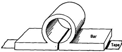
Fig. 4. Ring-core head: the ferromagnetic reproducing head of Fig. 2, modified to accept many turns of wire on a ring core, in order to increase the output voltage.
