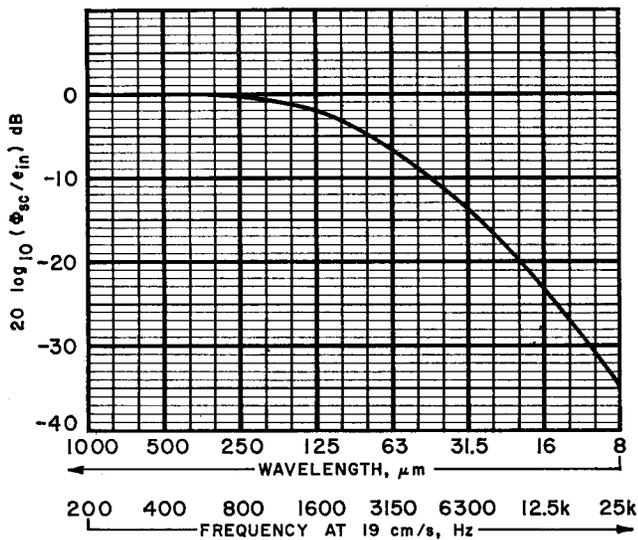
Fig. 6. An example of an unequalized recording flux-frequency response (the ratio of shortcircuit flux to the recorder input voltage vs. recorded wavelength).
