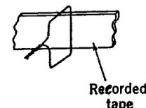
**Fig. 3. Single conductor non-ferromagnetic reproducing head.**
