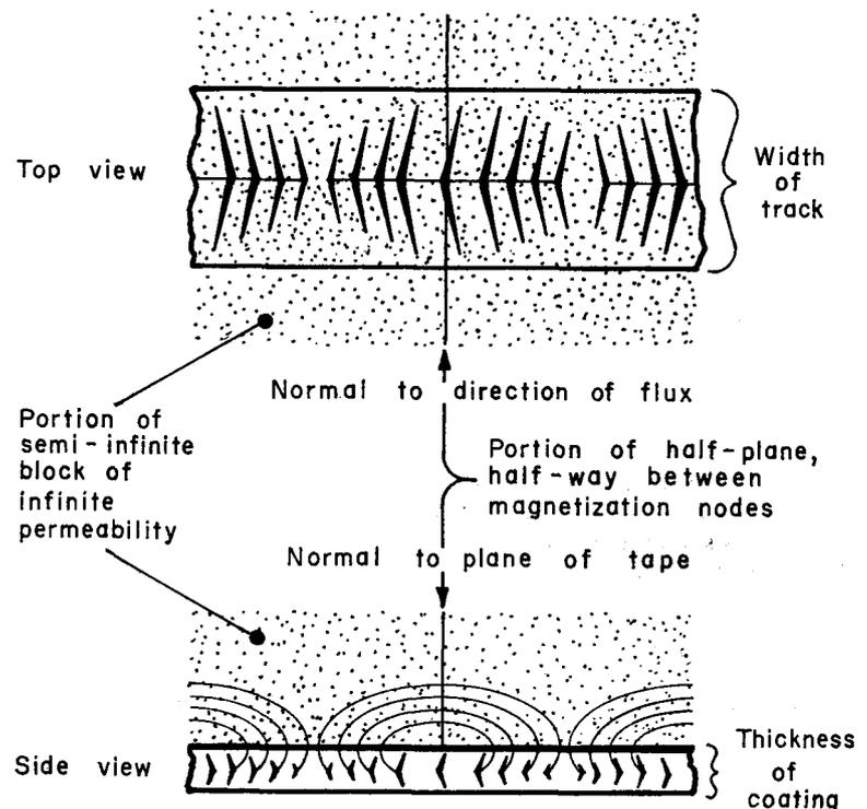
Fig. 10. Simplified illustration for the definition of "shortcircuit flux," showing the sinusoidal magnetization of the coating, the resulting flux, the relationship of the coating to the semi-infinite block, and the relationship of the flux to the half-plane of measurement. ("Half-plane" and "semi-infinite block" refer to the fact that they are bounded by the plane of the tape.)
