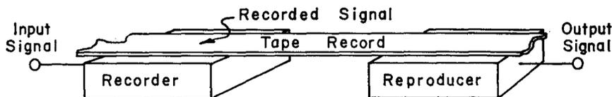
Fig. 1. Simplified recorder/record/reproducer system, showing the quantities needed for sensitivity and frequency-response specifications.
