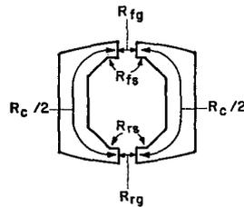
Fig. 5. Head-constructions for medium-wavelength measurement showing the flux paths and their reluctances: (a, left) the symmetrical head. (b, right) the high-efficiency head.
