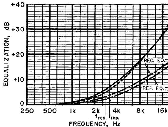
Fig. 8. Equalization at 19 cm/s (7.5 in/s): — total equalization required; - - - reproducer equalization, with transition frequency  $f_{rep} = 3150$  Hz; ···· recorder equalization, with transition frequency  $f_{rec} = 2800$  Hz; - · - total equalization from recorder and reproducer.
