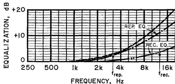
Fig. 7. Equalization at 38 cm/s (15 in/s): — total equalization required; - - - reproducer equalization, with transition frequency  $f_{rep} = 3150$  Hz; ···· recorder equalization, with transition frequency  $f_{rec} = 12.5$  kHz; - · - total equalization from recorder and reproducer.
